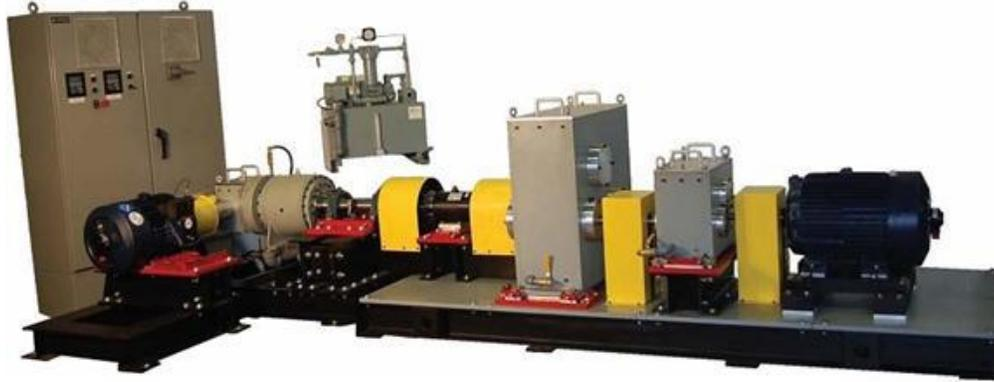
Figure 5. Planetary gearbox test rig [48]
