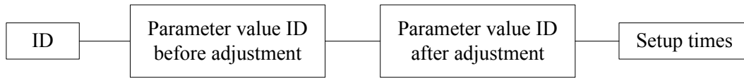
Figure 8 Data structure of the knowledge base of setup times of equipment parameters
