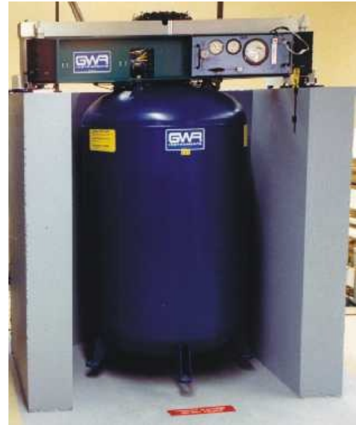
Canadian superconducting gravimeter in Cantley, Quebec
