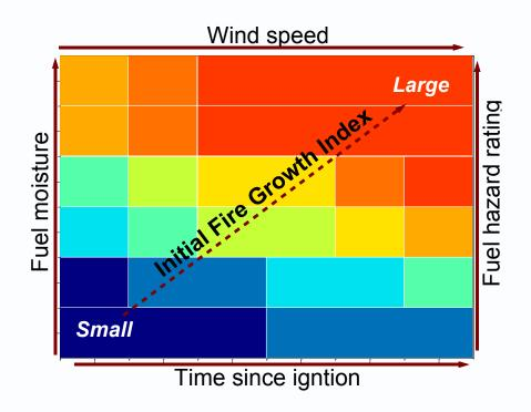
Conceptual diagram showing range of fire behaviour variables in developing a fire growth model or an Initial Fire Growth Index (IFGI) indicating the heightened potential fire size
