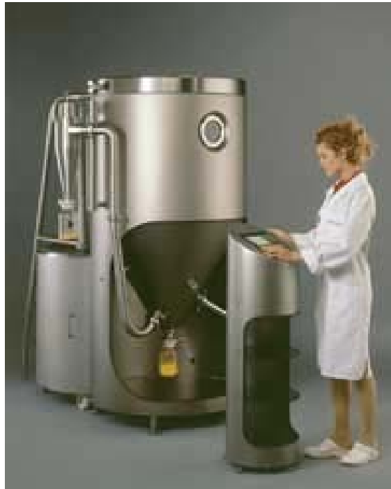
Niro Mobile Minor Evaporates 7 kg / h
