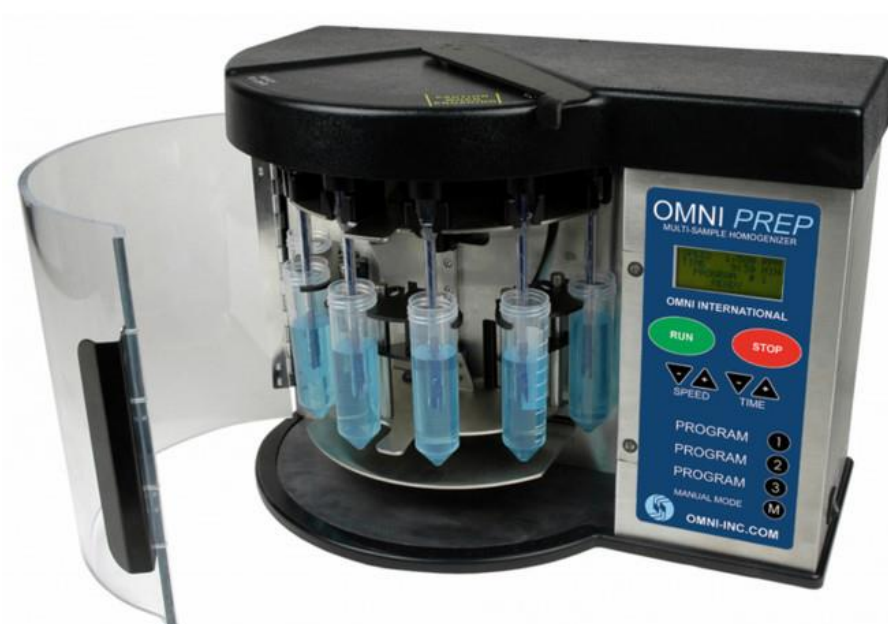
Lung samples removed, placed in 5 mL buffer, homogenized, centrifuged, and plated for assay of D29 and H37Rv levels (image from [8])
