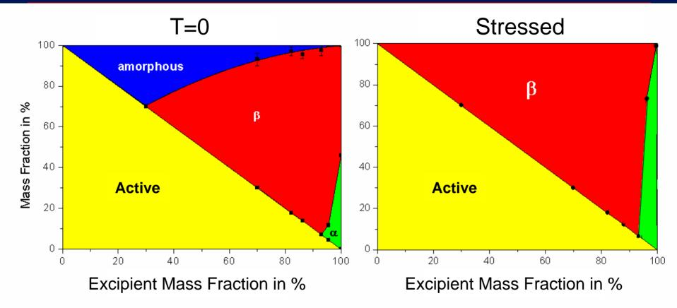
The method helps select formulations and processing conditions which lead to favorable solid state properties.
