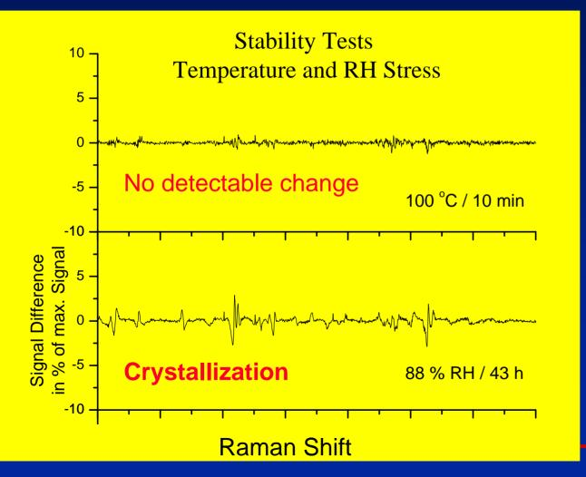
Excellent detection limits allowing early detection of stability problems
