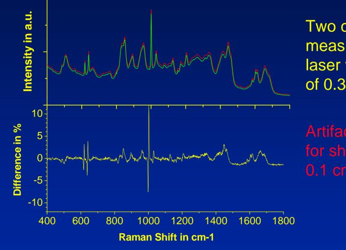
Two consecutive measurements with a laser wavelength shift of 0.3 cm<sup>-1</sup>
