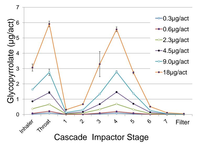
Glycopyrrolate cosuspension pMDls: Dose independent aPSD with linear FPM ( $r^2 = 0.995$ ) over a 60-fold dose range of 0.3-18 µg/actuation
