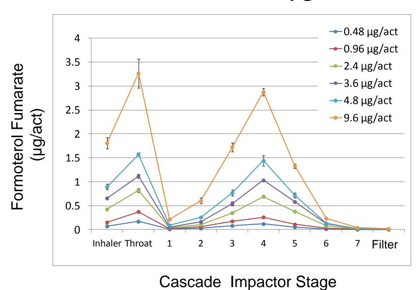
Formoterol fumarate cosuspension pMDIs: Dose independent aPSD with linear FPM ( $r^2 = 0.9997$ ) over a 20-fold dose range of 0.5 - 10 µg/actuation
