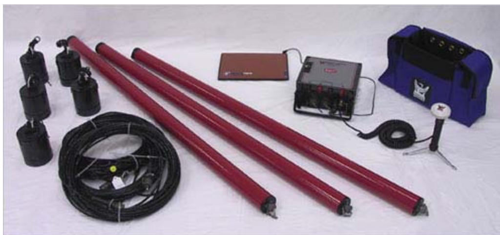
Figure 4-2. Phoenix V5-2000 MT system. From left to right; five non-polarizing electrodes, 3 induction coil cables, 3 MTC-50 induction coils, battery, recording unit, GPS antenna, case for the unit. Picture used courtesy of Phoenix Geophysics.
