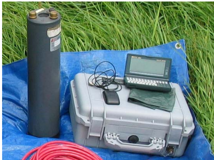
Figure 4-3. The NIMS MT system. From left to right; three component fluxgate magnetometer, sensor cable, GPS antenna and the data logger contained in the gray plastic case. Palmtop computer is used to control the data logger.
