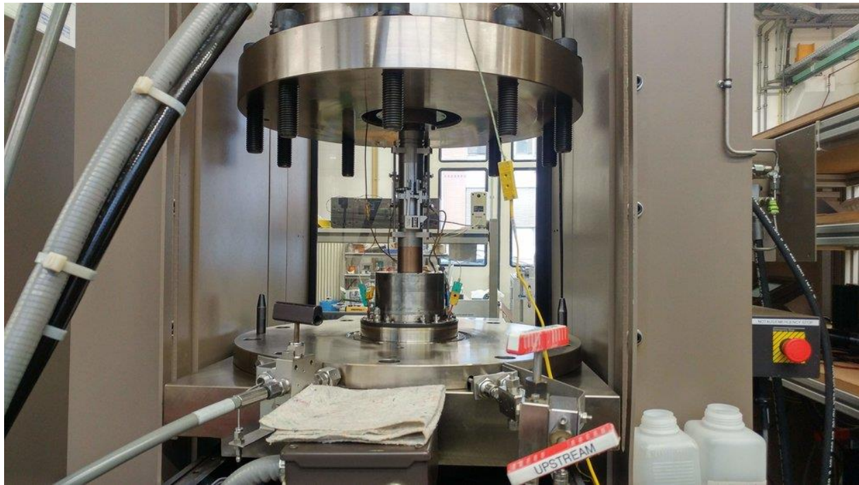
Figure A.50. Rock Mechanics Test System at the GFZ, used for determining behaviour of potential geothermal reservoir rock under stress.
