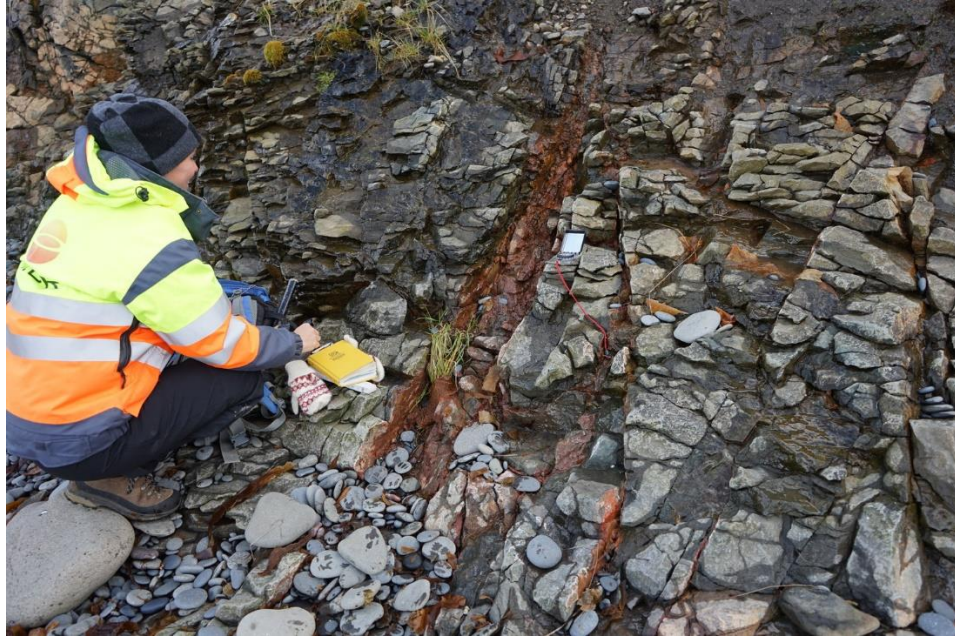
Figure A.28. Mapping north-south oriented fractures near Ytri-Vik. Red iron-staining suggests hydrothermal fluid circulation.
