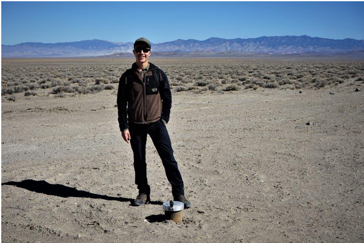
Figure A.35. A temperature gradient hole well head in Gabbs Valley. You wouldn't know it from the surface, but 117 m down this well, water temperatures reach 152 C!
