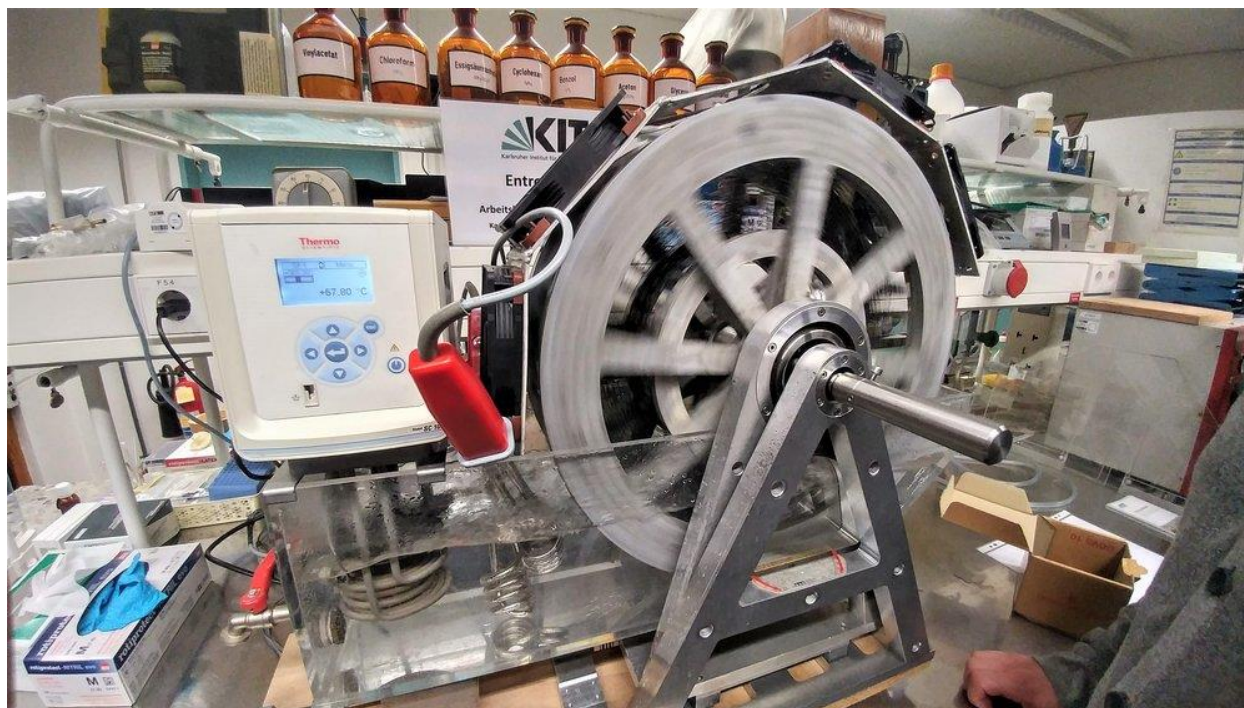
Figure A.45. Entropy wheel at KIT. In this image the wheel is rotating clockwise. The axis of the outer wheel is offset above and to the right of the inner wheel, driving continuous rotation. Note that the water temperature is <60°C!
