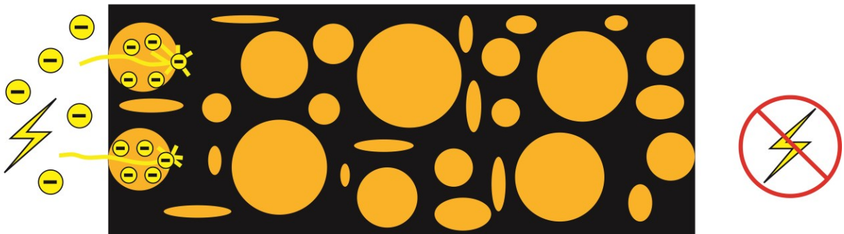
Figure 3.4: Conceptual model demonstrating the Hashin-Shtrikman upper and lower bounds and how they relate to the movement of electrical charges. \rho denotes the resistivity of the two materials (gold and black).
