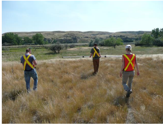
Photo 1: View from the terrace at the base of the cliff towards southeast, across the alluvial plain and towards the Milk River, which can be seen in the background. The EM31 is operated at hip height in VDM.
