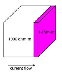
The sample has 10% porosity. This geometry represents a **series circuit**, and electric current cannot effectively bypass the resistive rock grains. It must travel through both the conductive liquid and resistive rock grains.
