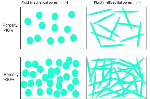
Note that the elongated pores will connect to form an interconnected electrical network at a lower porosity than the spherical pores. Is the permeability of the two cases different?
