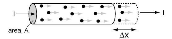
n = number of charge carriers per unit volume q = the charge on each carrier
