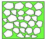
To compute the overall electrical resistivity, we must consider current flow through each phase. However, given the much higher resistivity of the grains, most current will flow through the water, with ions as the charge carriers.
