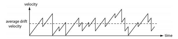
The ease with which the charge carrier can move is described by the mobility,  $\mu$ , which is defined as the drift velocity per unit electric field = v/E
