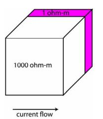
The sample has 10% porosity. This fluid geometry represents a **parallel circuit**, and electric current can effectively bypass the resistive rock grains and travel through the sample entirely in the conductive liquid.
