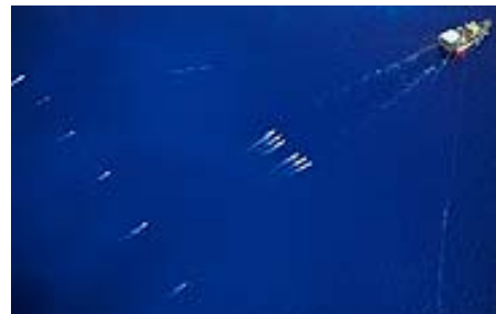
Airgun array and streamers being towed behind a survey vessel.
