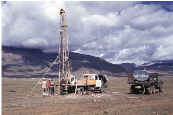
Drilling shot holes in Tibet, 1994
