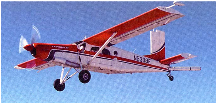
Aircraft mounted cesium vapour magnetometer
