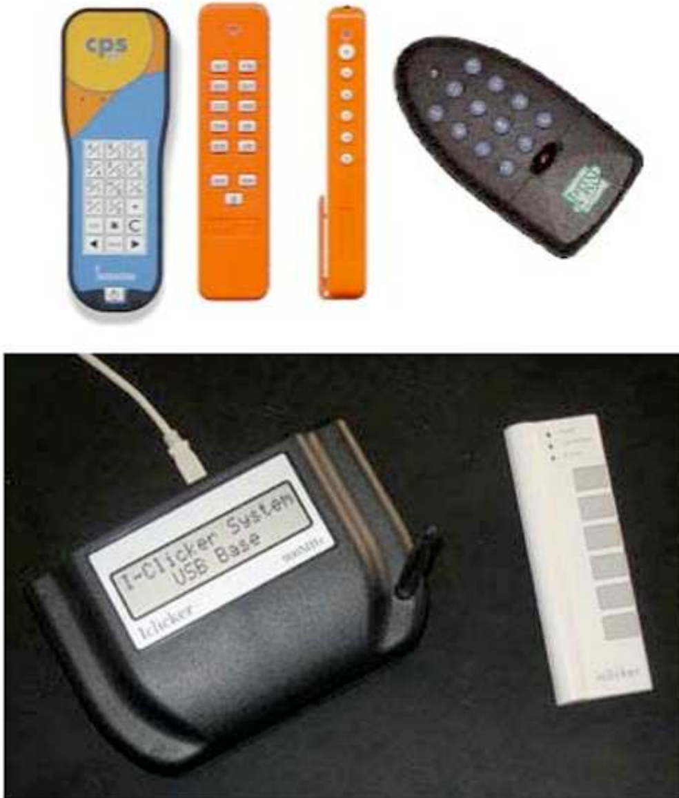
Figure 3. Infrared transmitters (top) and radio (RF) receiver and transmitter (bottom).
