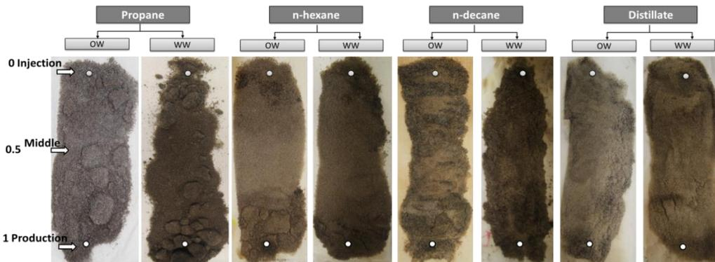
**Figure 5-3: Experimental sandpack after testing with different types of solvents and surface wet (water-wet and oil-wet) at 50 °C and 2068 kPa.**
