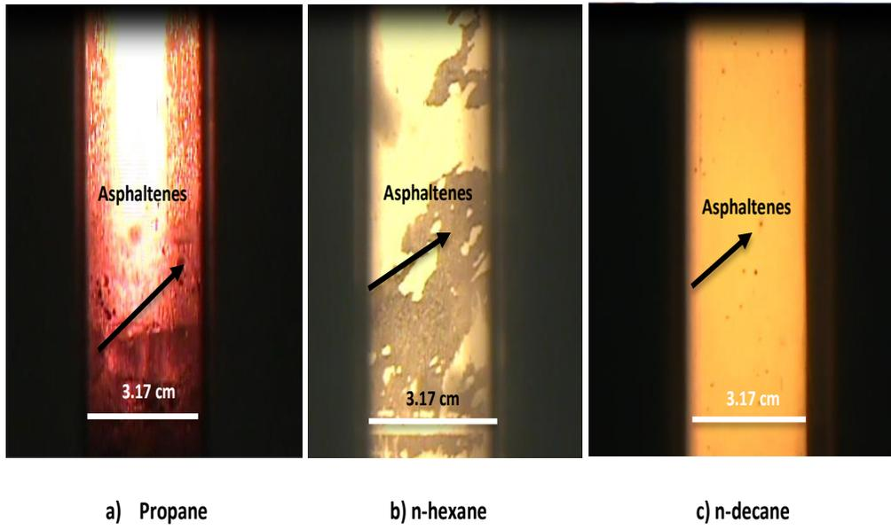
**Figure 2-13: Asphaltene concentration visualization in the PVT cell for different n-alkanes as precipitating agent at a constant volume ratio determined to be 5 cc solvent/1 g oil: a) C3 b) n-C6, c) n-C10.**
