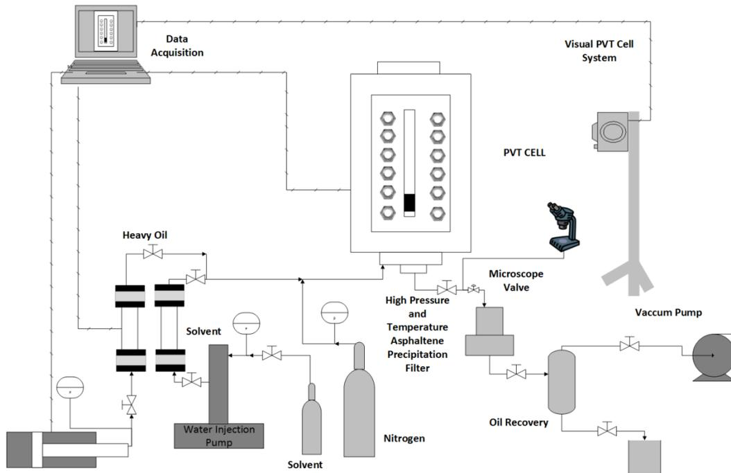
**Figure 2-3: Schematic flow diagram of experimental setup.**
