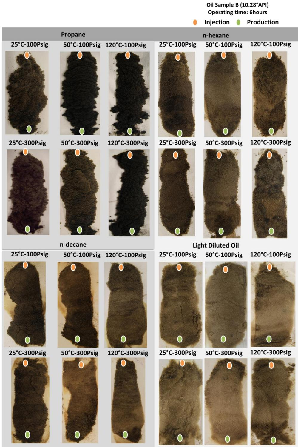
Figure 3-8: Sandpack after solvent injection (heavy oil A and B) using n-type solvent at different operational conditions and operational time (8-hour, oil A to 6-hour, oil B test). The vertical sandpack system has shown that high residual oil is present at the end of the production well.
