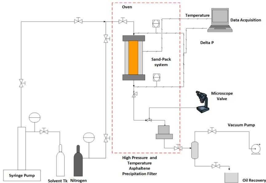
**Figure 3-3: Flow diagram of the gravity drainage recovery experiments on unconsolidated sands.**
