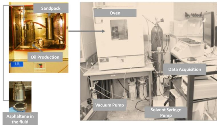
**Figure 3-4: Unconsolidated sandpack system setup - Physical model.**
