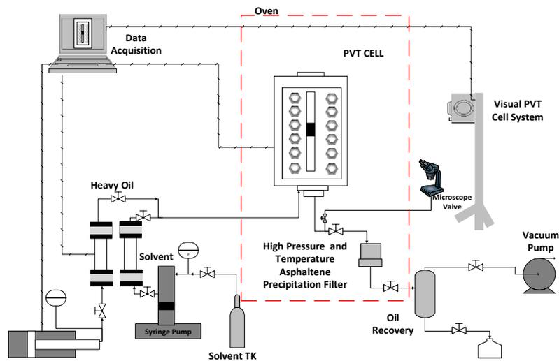
**Figure 4-3: Optical PVT cell: Asphaltene flocculation flow diagram setup.**
