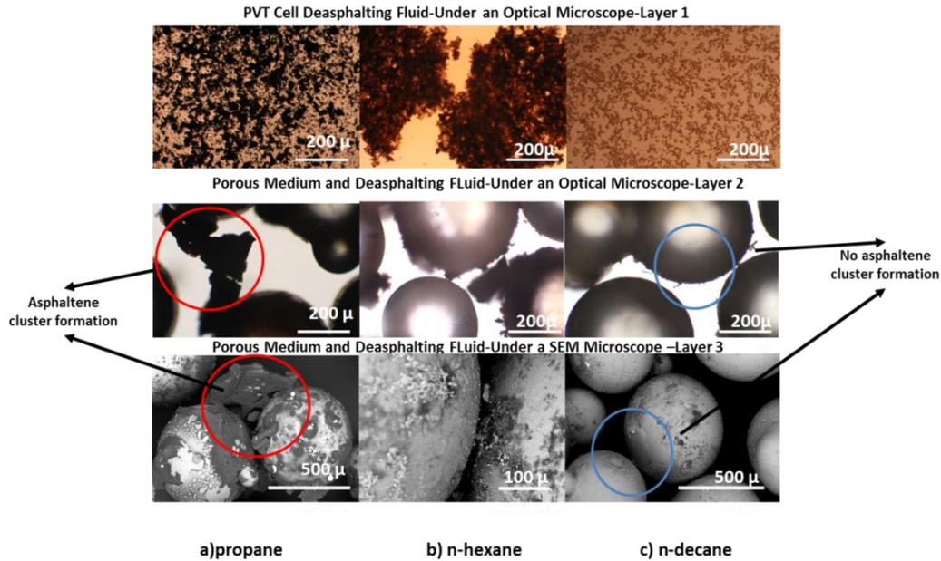
**Figure 2-7: Asphaltene deposition on the glass beads (porous medium test) (Moreno and Babadagli [40,41]) and asphaltene precipitation in the fluid (PVT cell experiments) after deasphalting with different n-alkanes: a) C3, b) n-C6 and c) n-C10.**
