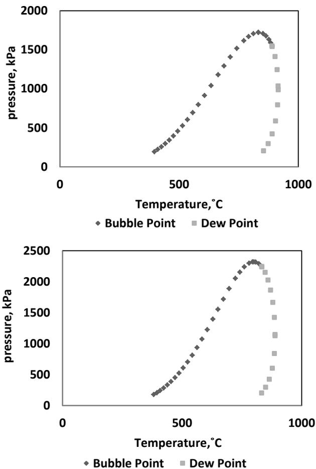
Figure 4-2: Heavy oil A and B envelopes from the dead oil.
