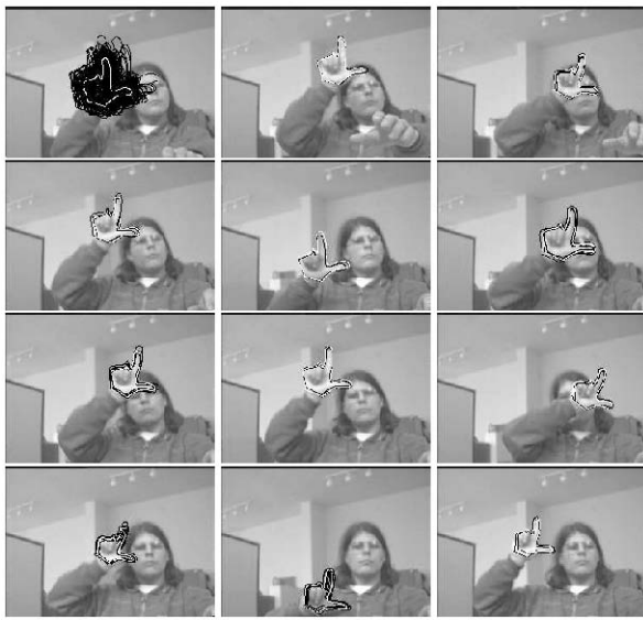
Figure 2. Tracking hand in clutter with 100 particles. Black contours show particles having high observation likelihoods, whilst the white contour shows the predicted contour of the hand.
