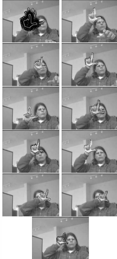
Figure 3: Tracking hand in clutter with 100 particles. Black contours show particles having high observation likelihoods, whilst the white contour shows the actual estimate of the hand.
