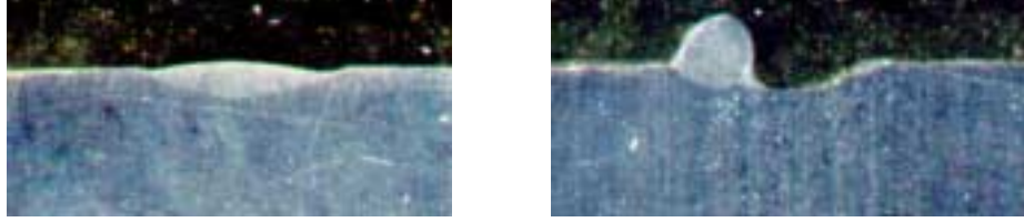
Figure 6-17: Comparison of penetration for high and low sulfur welds. The weld on the left has a sulfur content of 6 ppm and the one of the right 230 ppm. The penetration for both welds is 0.9 mm. The weld on the right showed a double humping defect, which appears as a bump.
