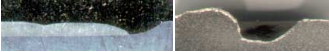
Figure 7-3: Contact angle for low and high sulfur. The sulfur content of the base metal is 6 ppm for the picture on the left, and 230 ppm for that on the right. It can be observed that the trailing region with higher sulfur content has a less wetting contact angle at the end of the gouging region.
