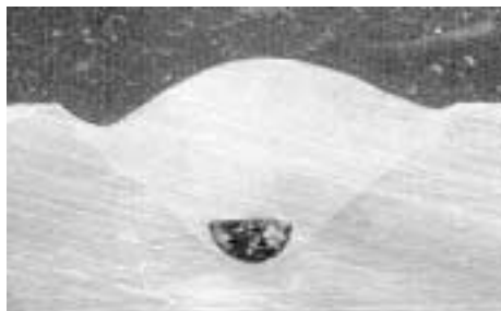
Figure 5-3: Tunnelling in GTAW. The cross section of the channel appears at the root of the weld. This weld was made with a current of 390 A and a travel speed of 12 ipm; the shielding gas was 98% Ar, 2% O 2
