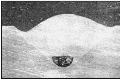
Fig. 3 — Tunnel porosity in GTAW.
