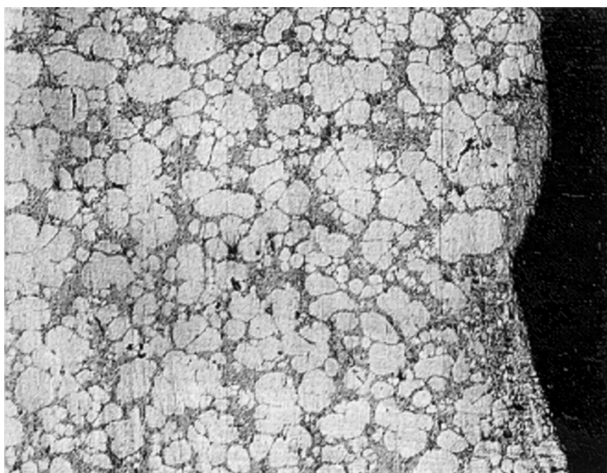
Figure 3 Cross section of joint between two semi-solid layers [3].
