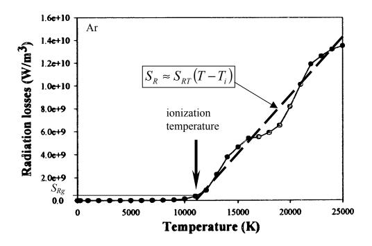
Fig. 4: Definition of ionization temperature. Argon plasma properties from [50]
