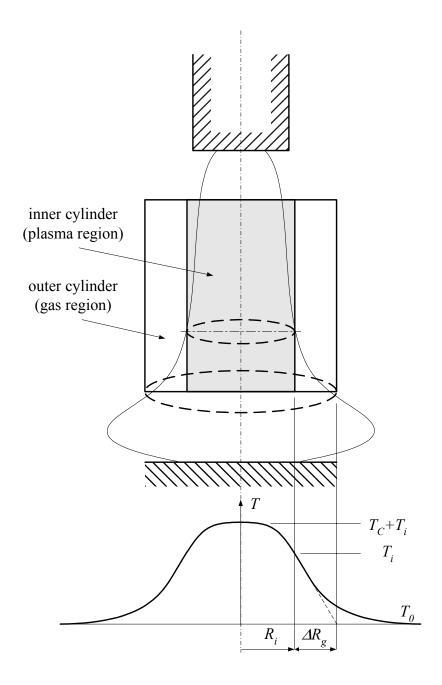
Fig. 3: Inner and outer cylinders containing the plasma and gas regions of the arc column
