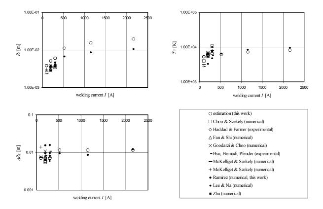
Fig. 6 Estimations and numerical calculations of  $R_i$ ,  $T_C$ , and  $\Delta R_g$ . In all cases the estimations predict the correct order of magnitude.
