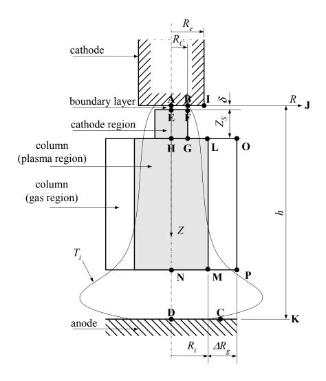
Fig. 1 - Long GTA welding arc , and its transition region. In a long arc the arc length (h) is significantly longer than the characteristic distance  $Z_S$
