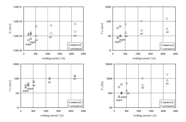
Fig. 5 - Estimations and numerical calculations of  $V_{RS}$ ,  $V_{ZS}$ ,  $P_{S}$ , and  $Z_{S}$ . In all cases the estimations predict the correct order of magnitude and functional dependence.
