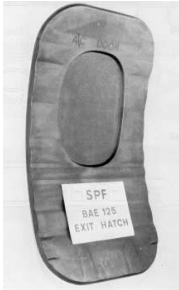
Figure 20 Exit hatch for the BAe 125/800 made of titanium SPF/DFW 33 .
