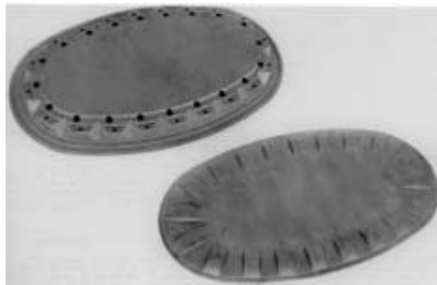
Figure 21 Wing access panel for the airbus A310/A320 made of titanium SPF/DFW 33 .
