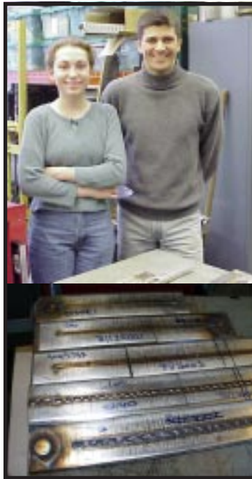
Sophomore Krista Niece (left) and doctoral student Patricio Mendez display welds (below) which show humping, supporting Mendez's order of magnitude welding model.
