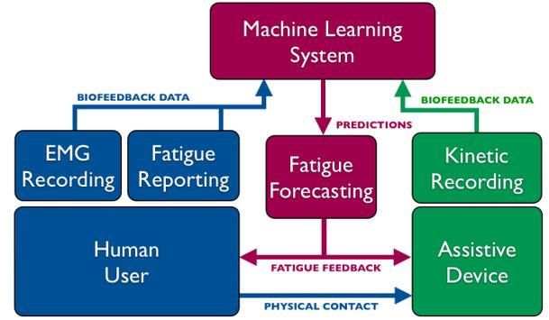
Fig. 1. A system to anticipate dangerous levels of muscle fatigue and provide user with temporally extended feedback about future exertion. Biofeedback signals are used to by a machine learning system to predict muscle fatigue; situation-dependent fatigue forecasting (feedback) can then be transmitted to the user and their device during real-time use and training to improve skill acquisition and help reduce the risk of injury during out-of-clinic use.
