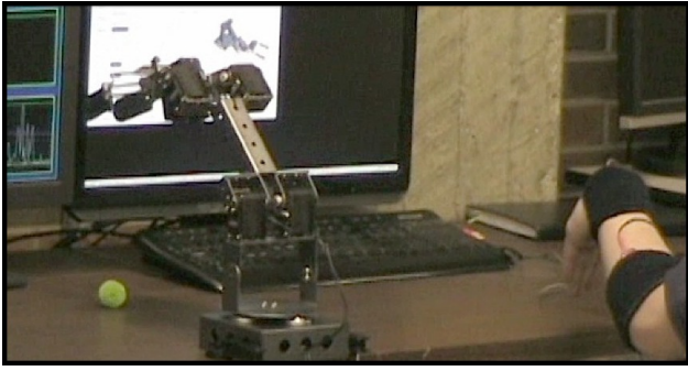
Fig. 2. Image of the AX-12 Smart Arm robot workspace and EMG setup.
