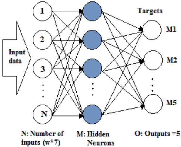
Fig. 3. Structure of the fully connected multi-layer perceptron neural network used for target prediction. The input data was the  $x, y, z$  coordinates of the environment-side robot end-effector, and the  $x, y$  coordinates of each eye. Window sizes ( $w$ ) of 4, 8, 12 or 16 samples of the input data were tested. The output layer had five output neurons, one for each mole.
