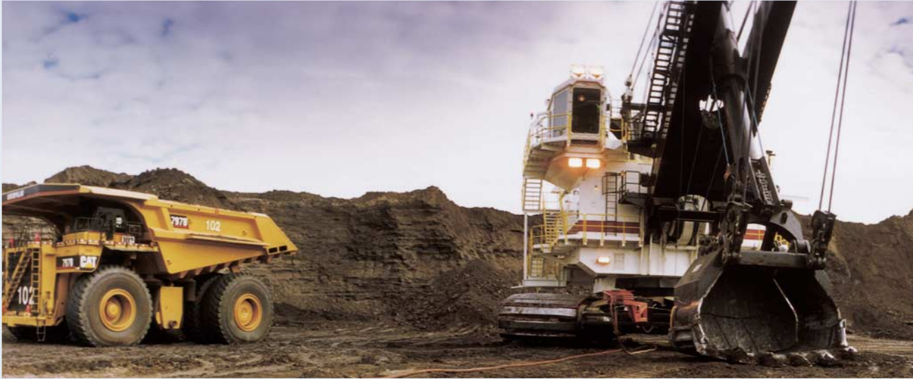
The world's largest haul truck, a Caterpillar 797B, and the first Bucyrus 495HF electric rope shovel in operation at the Muskeg River Mine.
