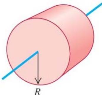
Thin-walled hollow cylinder
