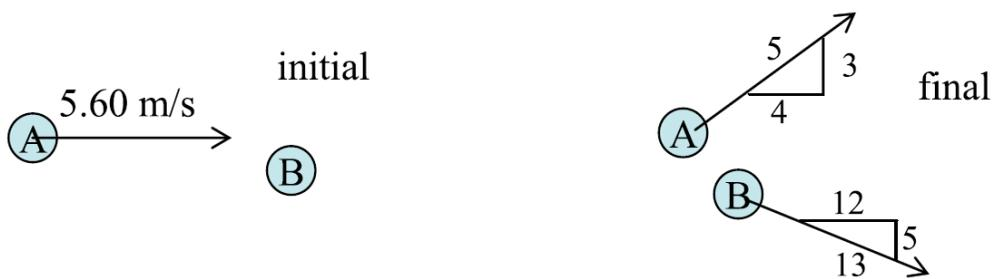
16. What is the speed  $v_{A2}$  after the collision?
