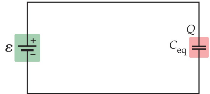
(b) Equivalent capacitance with same total charge
