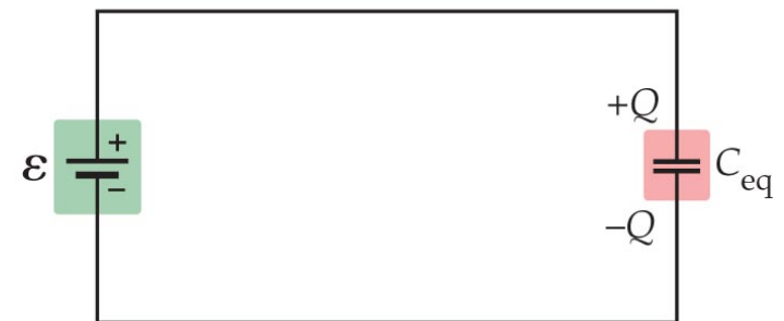
(b) Equivalent capacitance with same total charge
