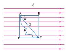
In this problem, you will be asked to use the given diagram (Figure 1) to calculate the work done by the electric field E on a particle of charge q and see for yourself whether that work appears to be trajectory-independent. Recall that the force acting on a charged particle in an electric field is given by F = E q. Recall that the work W done on an object by a constant force is
