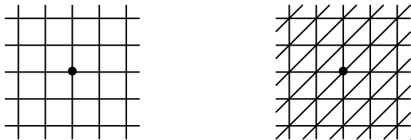
Figure: The quadrilateral mesh \mathbb{Z}_Q^2 (left) and the triangular mesh \mathbb{Z}_T^2 (right).
