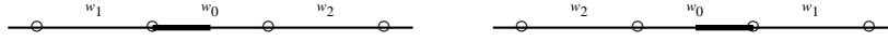
Figure 2: The 0-stencil (left) and the \frac{1}{2} -stencil (right) of the dual subdivision scheme in Example 2, where w_0, w_1, w_2 are given in (7). The \frac{1}{2} -stencil is the same as the 0-stencil. The value [\mathcal{S}_{a,2}v](k) for k \in \mathbb{Z} is attached to the center \frac{k-1}{2} of the line segment [k-1, k] instead of the vertex \frac{k}{2} . Since M = 2 , each line segment is equally split into two.
