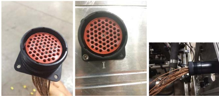
**Figure 2.22:** Thermocouple wiring (photo by author).
