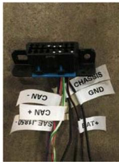
**Figure 2.21:** OBDII connector wiring (photo by author).
