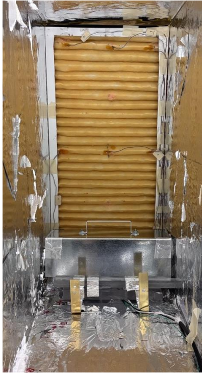
Figure 5.43. Aluminum frame cover used to stabilize the ceramic heater temperature before exposing the filter.
