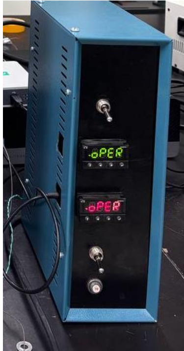
Figure 3.6. PID temperature controller used in the experimental setup.
