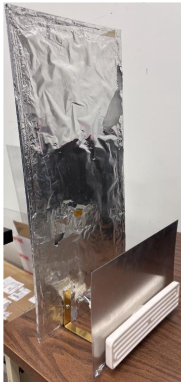
Figure 3.3. Ceramic heater setup with an aluminum reflector mounted on the gate to intensify forward radiation and reduce heat dissipation.
