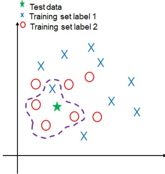
Figure 4.2: KNN schematic for 4-nearest neighbors. The algorithm labels the test data based on the labels for the 4 nearest neighbors.
