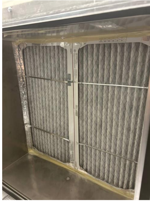
Figure 4-3- Two side-by-side filters installed in the wind tunnel
