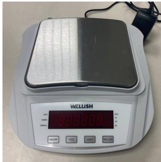
Figure 3-5- The scale used in particle release tests
