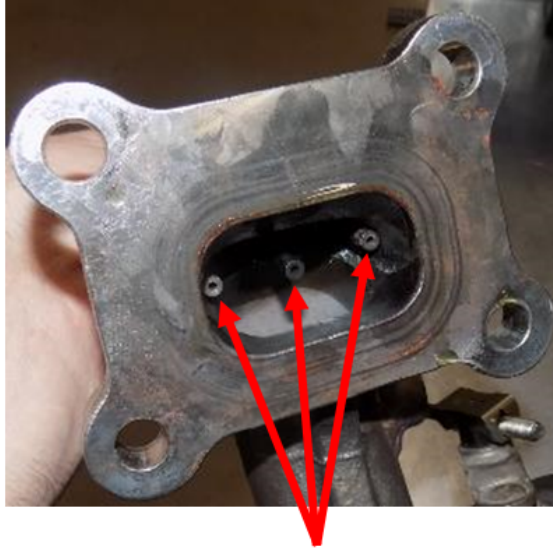
CO/CO 2 , HC, and NO x fast analyzer's sampling probes tips located at the outlet of the exhaust manifold
