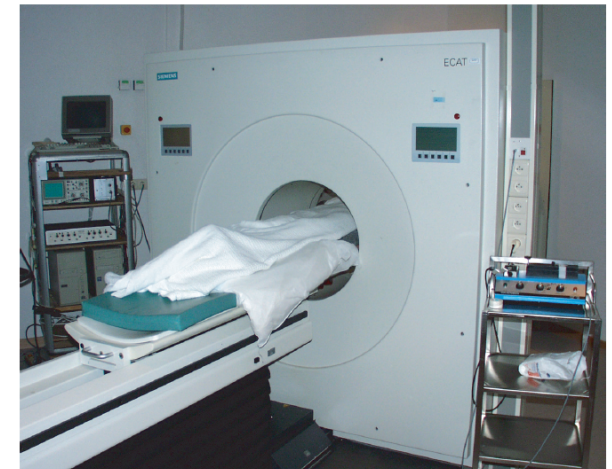
Figure 5.13 PET scanner. A movable table shifts the patient through the circular hole in the gantry. The external design is similar to that of a CT scanner and to some extent to that of an MRI scanner. (Courtesy of the Department of Nuclear Medicine.)
