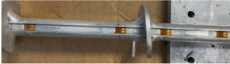
Figure A 5. Installed bending strain gauges.
