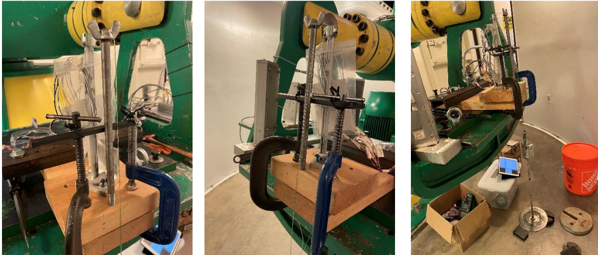
Figure A 6. Bending strain gauge calibration setup
