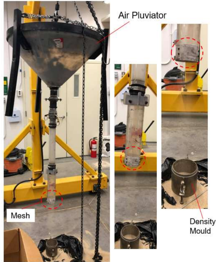
Figure 8. Calibration Assembly for the Portable Travelling Pluviator
