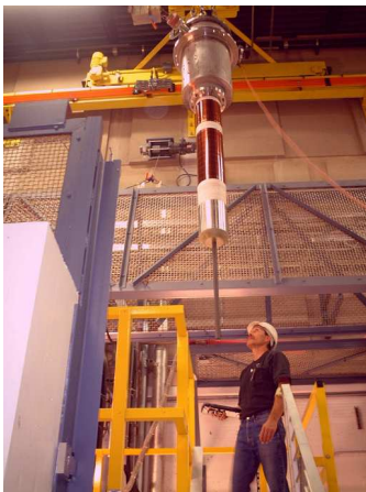
Figure 1. Insert magnet in transit to assembly inside 100 T outer magnet assembly
