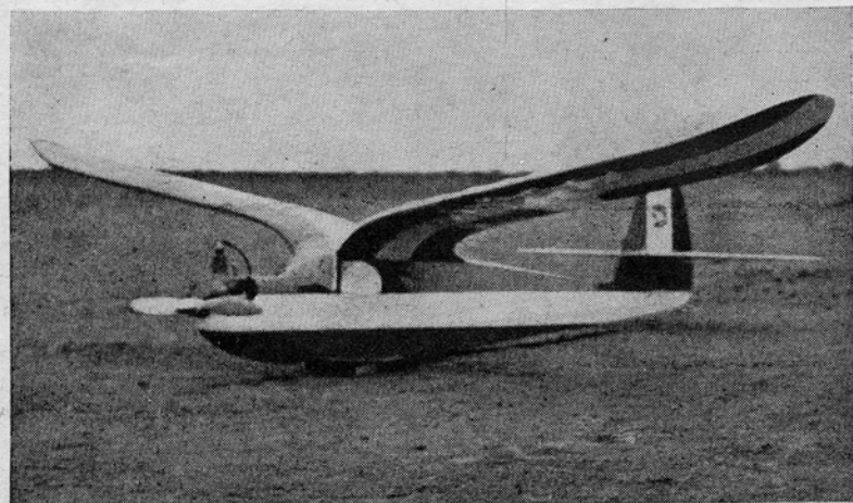
The model has a glide like a sailplane. The ship rolls almost to a standstill before even a wing-tip skid touches the ground. No ground loops, either!
