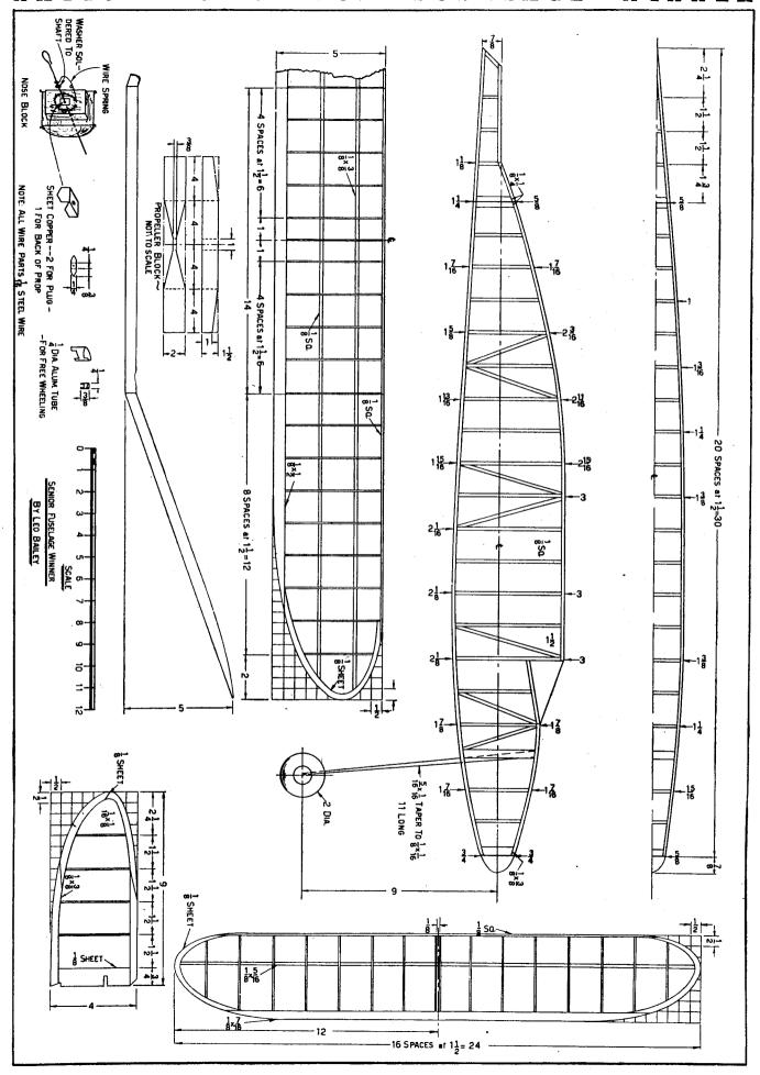
device which is exactly the same as Albert Judge used on his 1936 Wakefield Winner. Setting the wing at the angle of 4 already puts it practically at the angle it will fly, and makes excessive down-thrust unnecessary. Using the rubber tensioner allows an excessively long motor without the necessity of a long, unwieldy and ugly fuselage.
