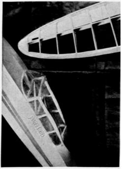
Here you see how the wing is constructed and details of the cabin construction
