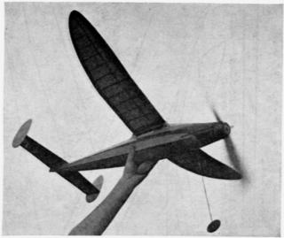
The twin rudders and large stabilizer provide great stability and soaring capacity
