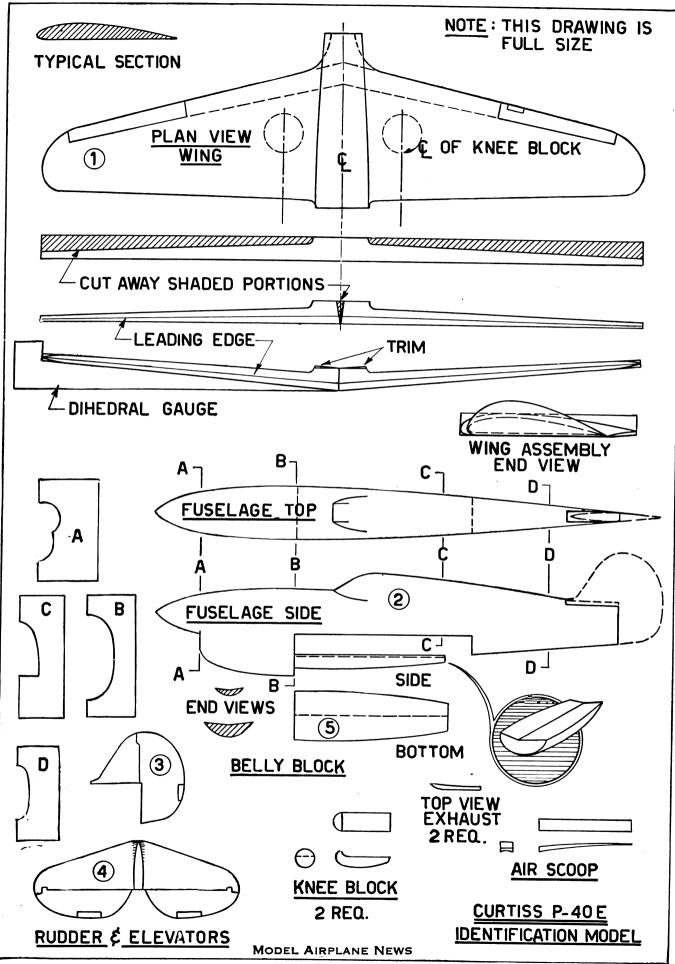
Tapering the wing and setting the proper dihedral angle is clearly illustrated in the drawings. First outline the front view of the wing as indicated in the plans.
