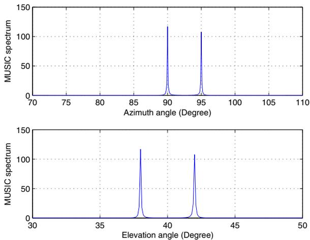
Fig. 7. Example 2: MUSIC spectrum for MIMO radar with 2D transmit beamforming projected onto the azimuth (top) and elevation (bottom) axes.
