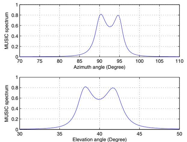
Fig. 5. Example 2: MUSIC spectrum for conventional MIMO radar projected onto the azimuth (top) and elevation (bottom) axes.
