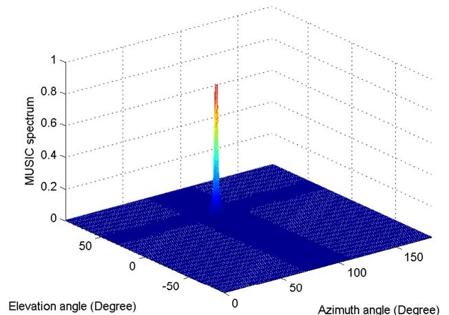
Fig. 4. Example 2: 2D MUSIC spectrum for conventional MIMO radar.
