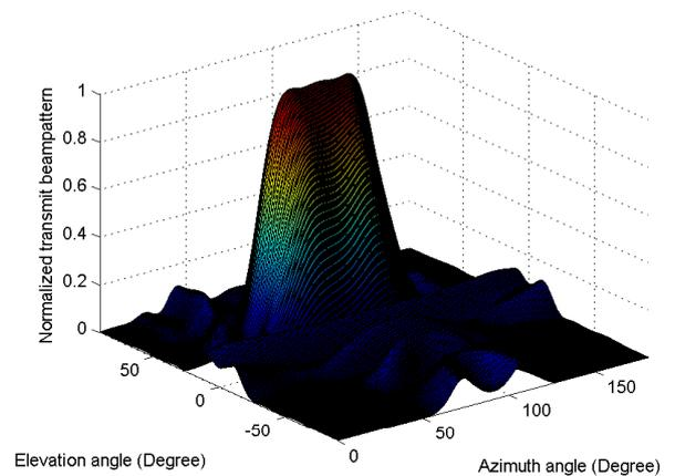
Fig. 2. Example 1: Normalized 2D transmit beampattern.
