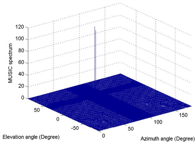
Fig. 6. Example 2: 2D MUSIC spectrum for MIMO radar with 2D transmit beamforming.
