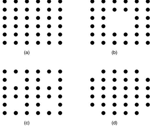
Fig. 1. Symmetric planar array configurations: (a) Uniform rectangular array (URA); (b) Uniform rectangular frame array (URFA); (c) Symmetric array with dual invariance structure; (d) URA with no elements at corners.
