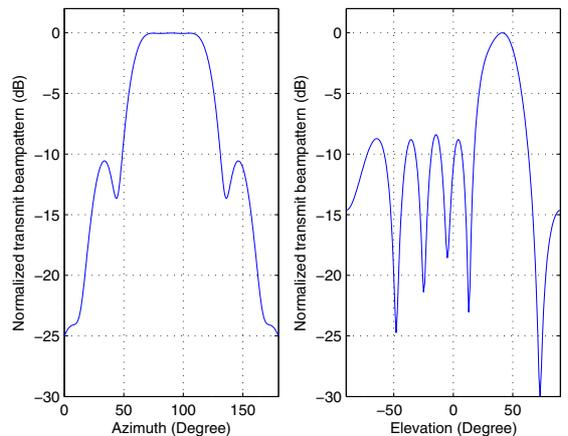
Fig. 3. Example 1: Azimuth and elevation cross sections of the normalized transmit beampattern calculated at  $\theta = 40^\circ$  and  $\phi = 90^\circ$ , respectively.
