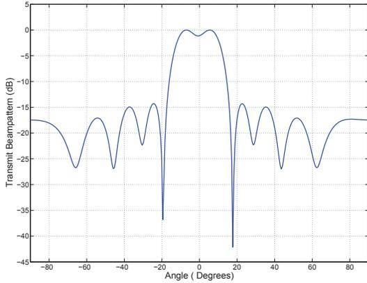
Fig. 1. Transmit Beampattern versus angle  $\theta$ .
