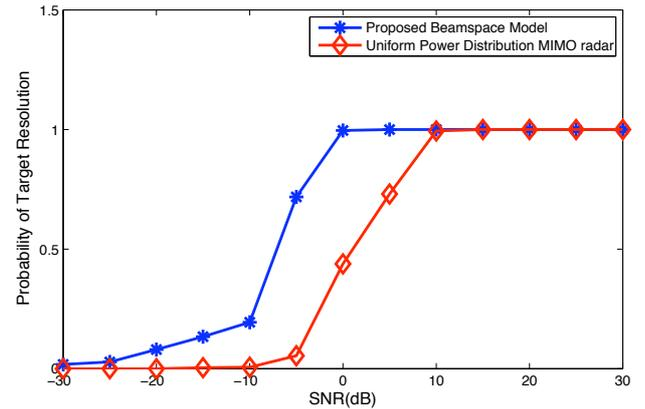
Fig. 3. Probability of resolution versus SNR
